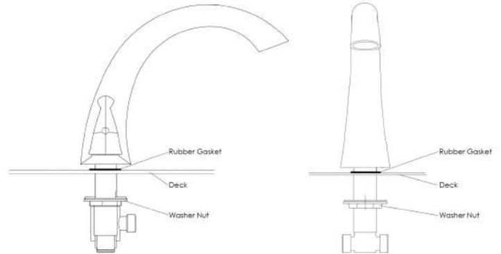
**2.** Unscrew the washer nut and place the rubber gasket and spout above the deck. After, secure the washer nut from underneath the deck.
